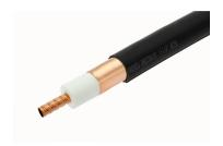
RCT6, RADIAX® Coaxial Radiating Cable with Bump, 70–960 MHz, tuned foil, 1-1/4 in, black non-halogenated, fire retardant polyolefin jacket
