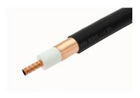
RCT6, RADIAX® Coaxial Radiating Cable with Bump, 50–3800 MHz, tuned foil, 1-1/4 in, black non-halogenated, fire retardant polyolefin jacket
